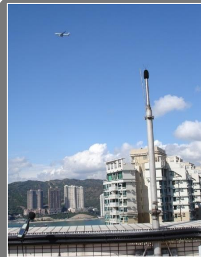
Figure 2-4: Outdoor noise monitoring terminal
