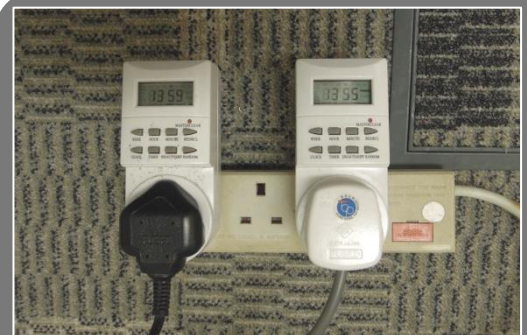
Figure 5-4: energy-saving timer devices connected to photocopiers
