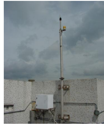
Figure 2-3: Outdoor Noise Monitoring Terminals
