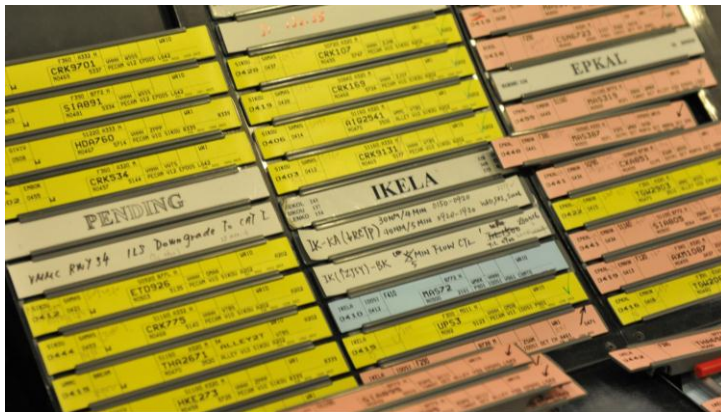
Figure 4-4: Traditional paper flight progress strips
