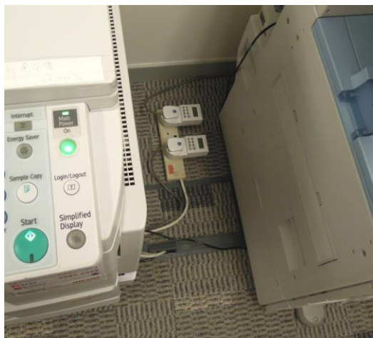
Figure 5-10: (Left) Energy-saving timer devices connected to the photocopiers and (Right) an the energy-saving timer device
