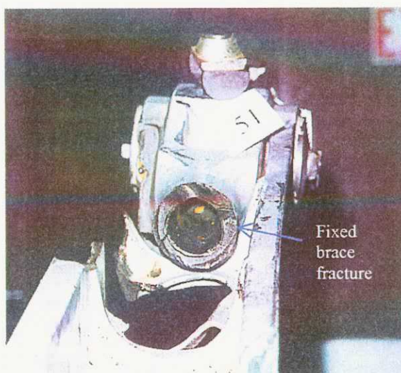
Figure 24. Outboard end of the fixed brace from Ship 518 (China Airlines) [left]
