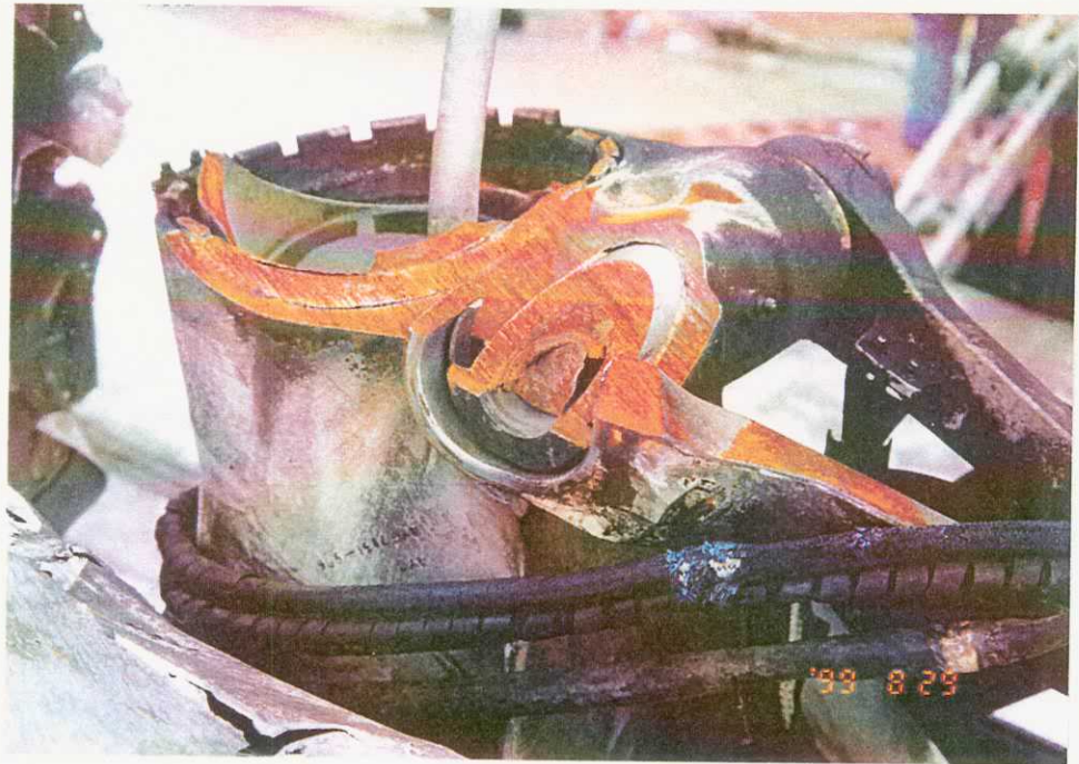
Fractured Center Landing Gear Oleo (Figure 13)
