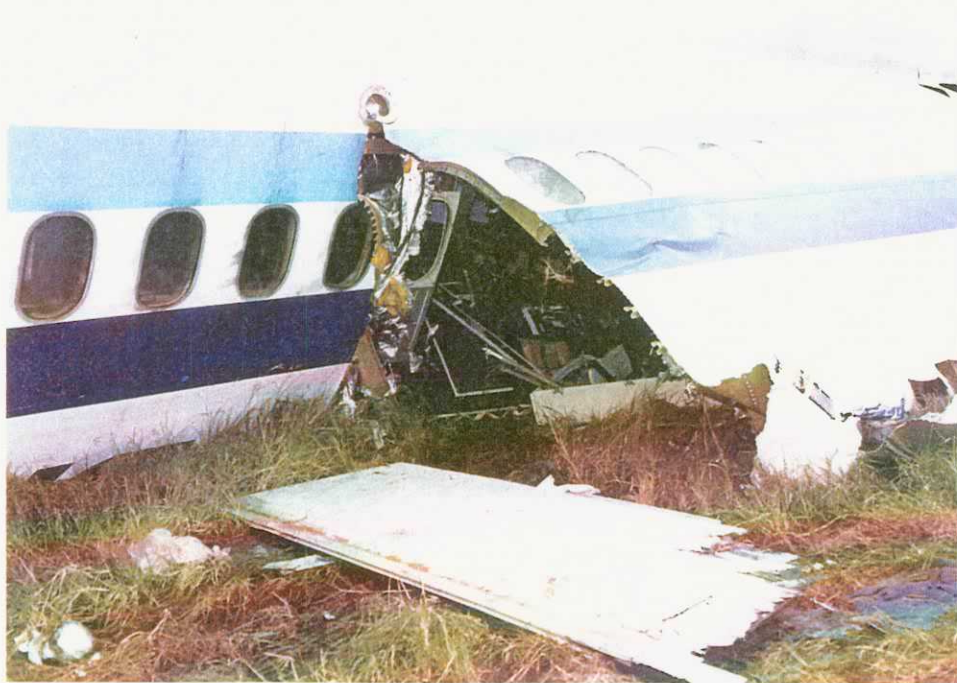
9. View of crack in right fuselage (aft).
