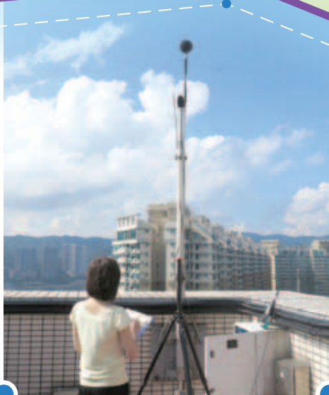
技術行政組人員正在收集飛機噪音數據。 An officer of the Technical Administration Section collecting aircraft noise data.
