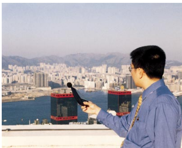
在中環量度飛機噪音水平。 Measuring aircraft noise levels in Central.
