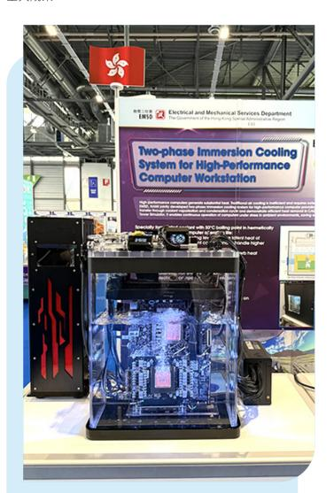
The award-winning two-phase immersion cooling system for a high performance computer workstation 獲獎的的高性能電腦工作站兩相浸沒式冷卻系統
