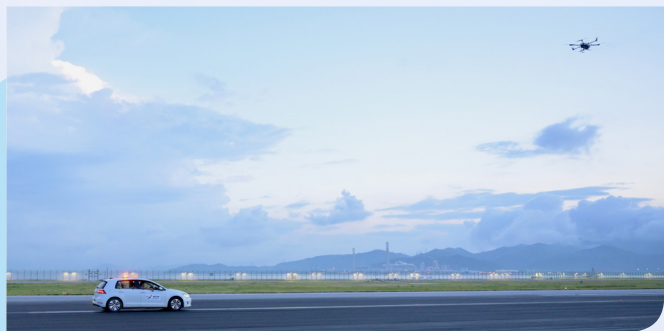
Photo shows the SUA of the trial flying along the centre line over the North Runway to inspect the signals emitting from the ILS.
