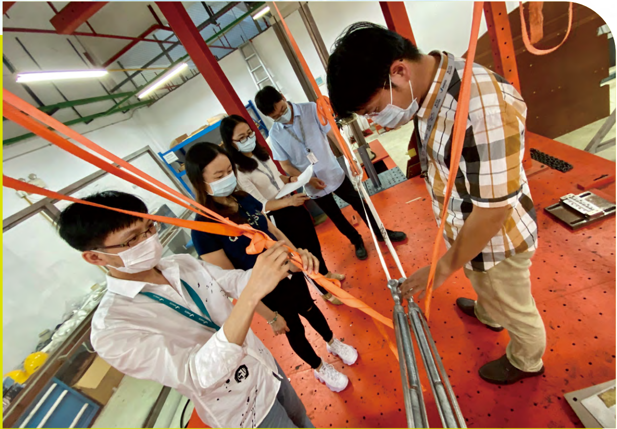
Structural testing of cargo restraint system 對貨物繫留固定裝置進行結構測試
