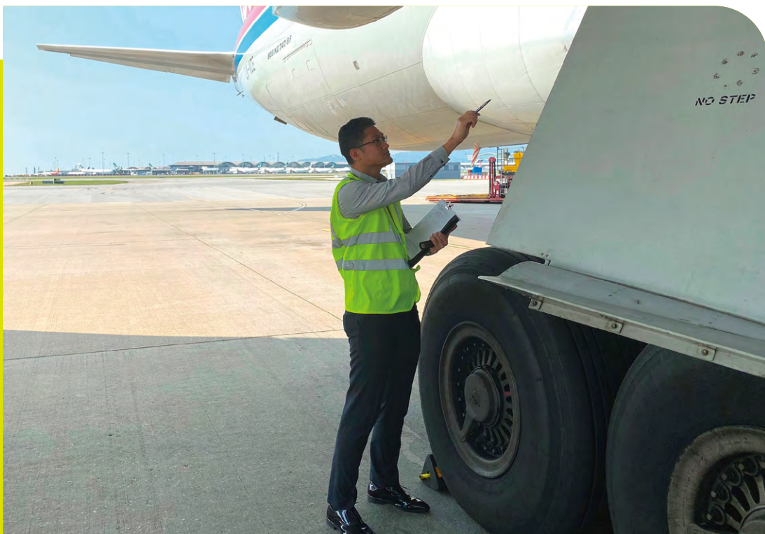
Inspector from the Flight Standards and Airworthiness Division inspects a foreign registered aircraft at the HKIA under the SAFA inspection programme. 飛行標準及適航部的督察根據 SAFA 檢查計劃，在香港國際機場檢查一架外地註冊的飛機。
