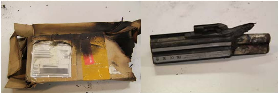
Figure 3 – Fire damage of an undeclared lithium ion battery for computer
