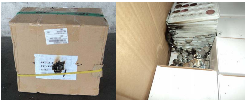
Figure 2 – Short circuit and the resulting fire damage of an undeclared package of lithium metal button cells
