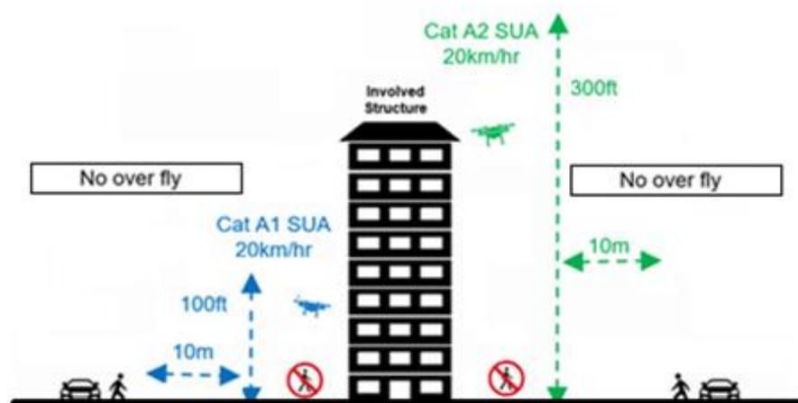
Figure 1: Building survey/ inspection under Standard Operations
