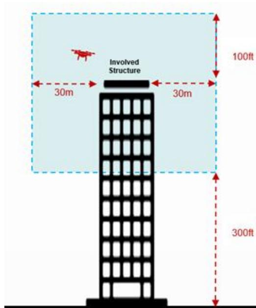
Figure 2: The pre-defined flight volume for high-altitude building survey/ inspection
