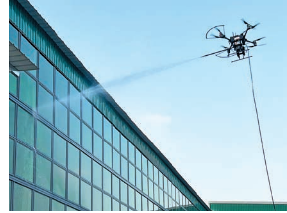
◆ 測試使用無人機清潔窗戶。 Testing of window cleaning by unmanned aircraft.
