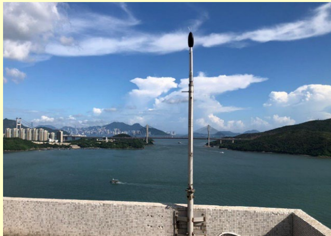
Figure 2-4: Outdoor noise monitoring terminal
