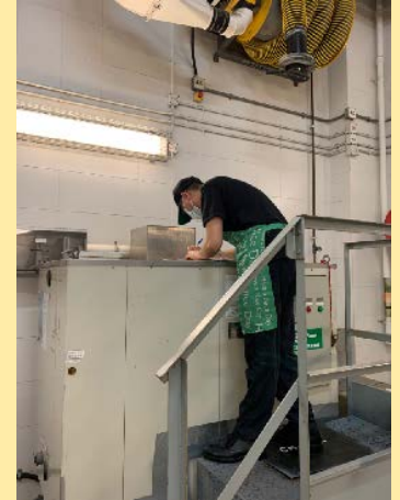
Figure 5-10: Operation of the food waste decomposition system in CAD Headquarters
