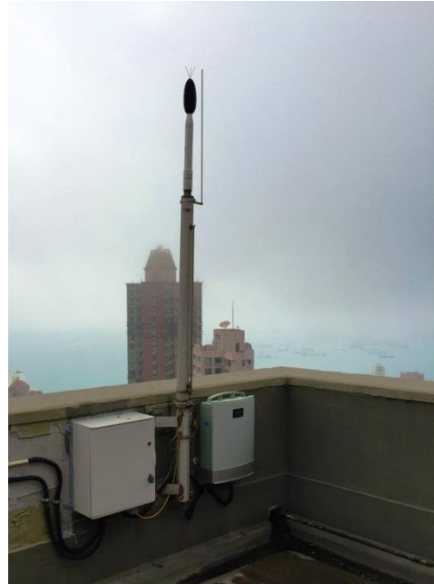
Figure 2-5: Outdoor noise monitoring terminal
