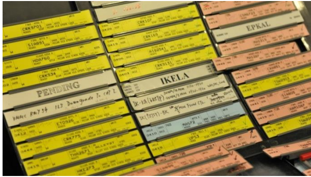
Figure 4-1: Traditional paper flight progress strips
