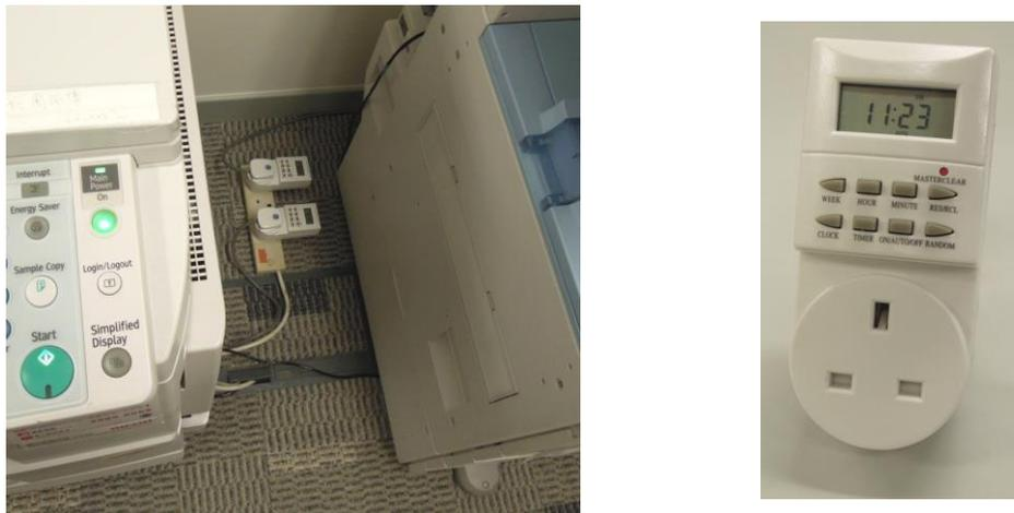
Figure 5-1: (Left) Energy-saving timer devices connected to the photocopiers and (Right) an energy-saving timer device
