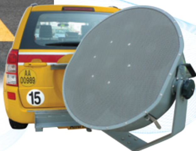
為防止航機受鳥擊影響，機管局購置遠距離揚聲裝置驅趕雀鳥。 A long range acoustic device for bird deterrence procured by AAHK to prevent bird strike.
