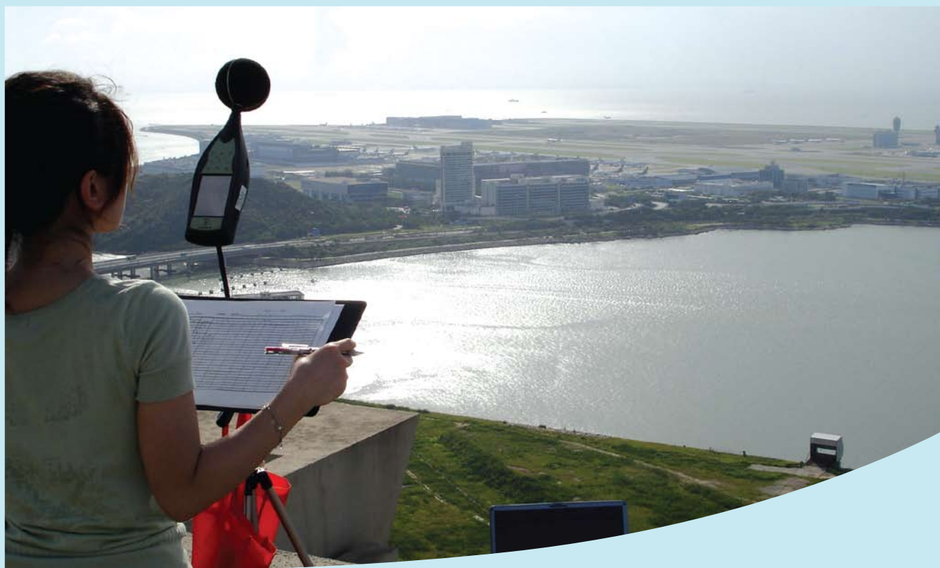
民航處人員正在收集飛機噪音數據。 An officer collecting aircraft noise data.
