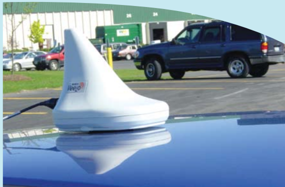
改進型地面活動引導和控制系統的車輛應答機。 Vehicle Locator for Advanced Surface Movement Guidance and Control System.
