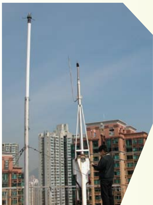
本處人員正在收集飛機噪音數據。 An officer collecting aircraft noise data.
