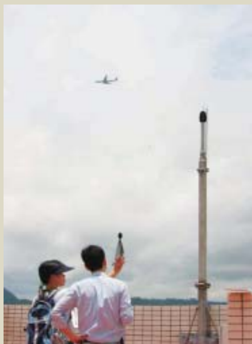
精密的噪音監察儀器可測量航道下民居受飛機噪音影響的情況。 Aircraft noise impact on residential areas under the flight path is measured by sophisticated noise monitoring equipments.
