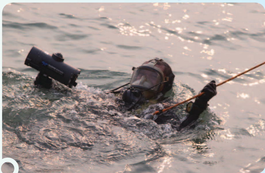
Diver with handheld acoustic receiver starting the homing search. 蛙人手持手提聲波接收器開展搜索。
