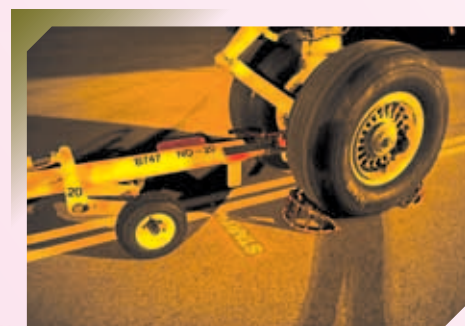
Ground marking for Aircraft Pull 拉飛機地面標記
